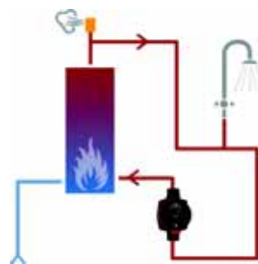
Fig. 6 Domestic hot-water recirculation system
