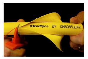
**REMOVE OUTER COVER:** Following the score around the circumference of the pipe, fully remove the section of outer secondary cover. Closely inspect the internal primary cover to ensure it has not been penetrated adjacent to the outer secondary cover. Cut off any excess cord exposed when the cover has been removed.
