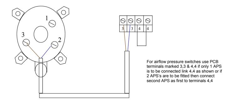
Airflow switches (mechanical installation)
