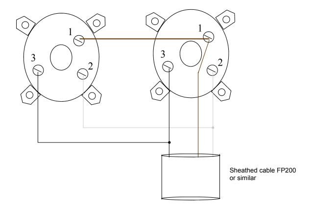
With the above wiring layout you would connect the grey and black into air pressure switch terminals 3 & 3 on the PCB as normal. These connections would in effect be the actual interlock.
