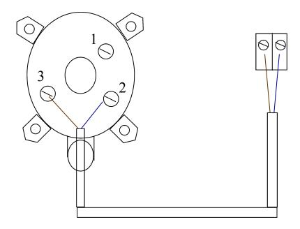
For airflow pressure switches use PCB terminals marked either intake or extract fan, these interlocks have a time delay in the software to prevent the effects of pressure switch flutter
