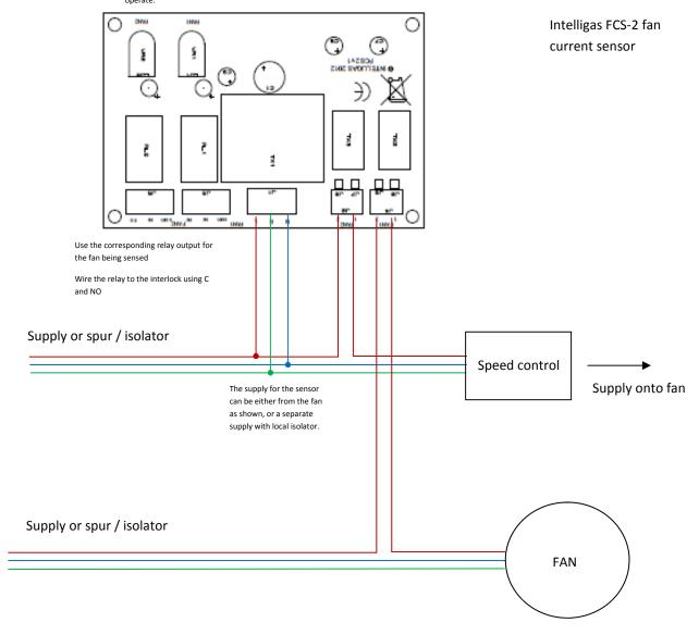
If the fan is 3 phase then divert one of the phases only through the current sensor.
