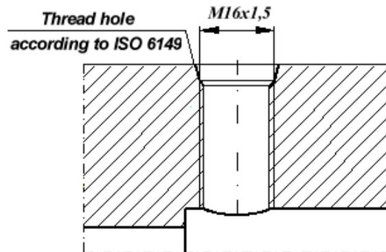
Figure 8: Assembly hole for the HF-pulse sensor HF3 in the meter body
