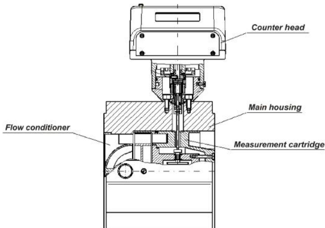
Figure 2: Sectional view of the industrial quantometers CPT
