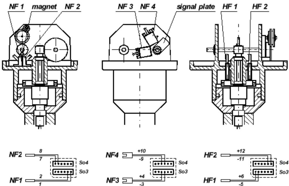
Figure 6: Position of the NF and HF pulse sensors in the counter head of the quantometer CPT
