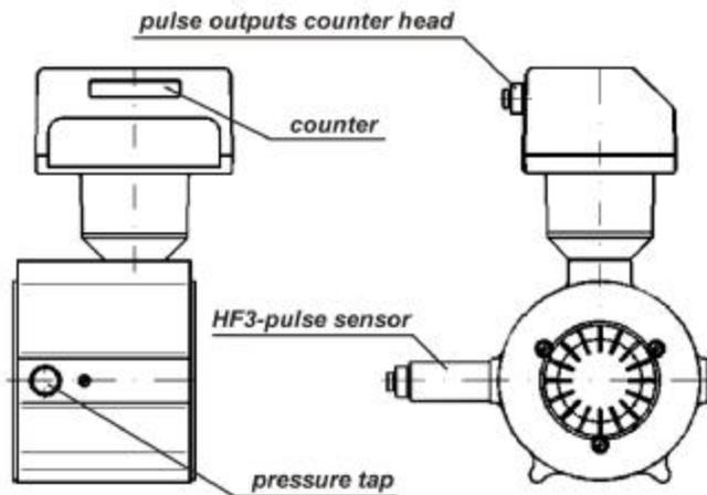
Figure 3: Measurement outputs of the industrial quantometer CPT
