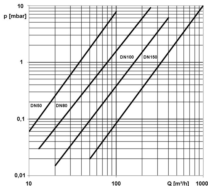
Figure 19: Pressure loss diagram of the quantometer CPT of a density  $\rho_0 = 1\text{kg/m}^3$
