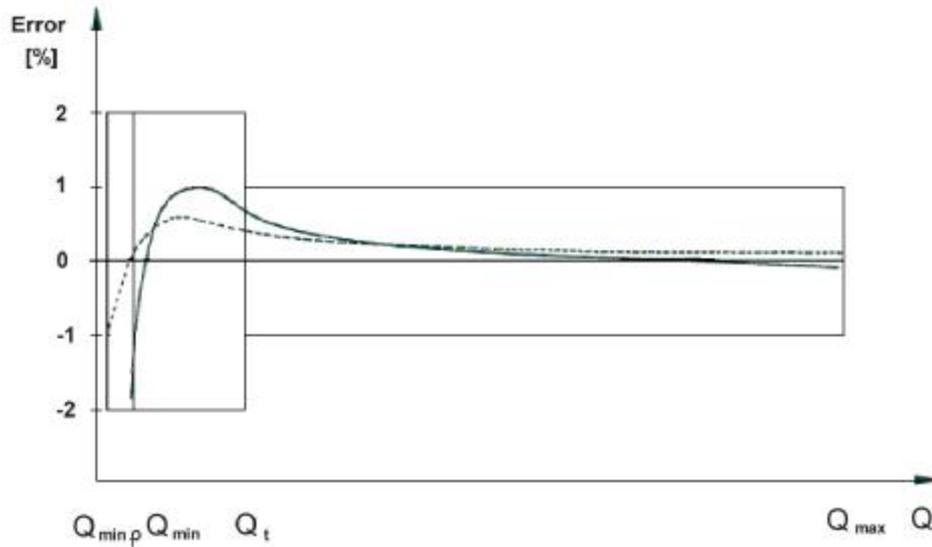
Figure 18: Error characteristic of a quantometer
