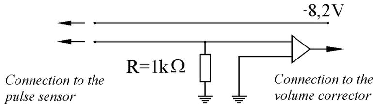
Figure 9: Diagram of connections of the inductive NAMUR initiators
