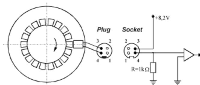
Figure 5: Pattern of the connector of the HF pulse sensor HF3 in the meter body
