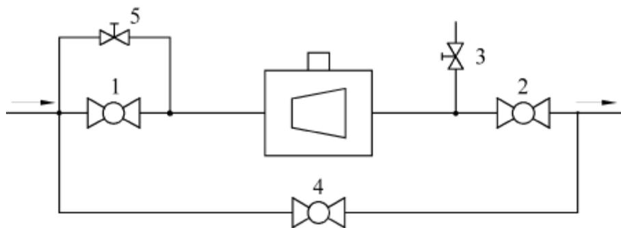
Figure 20: Pattern of a measuring system with bypass
