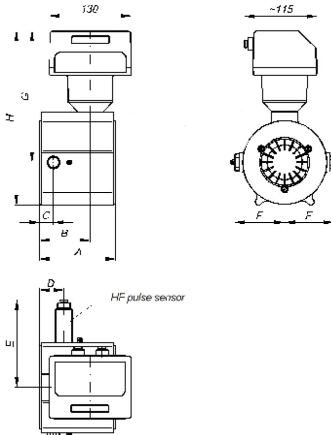
figure 1: External dimensions of the industrial quantometer CPT
