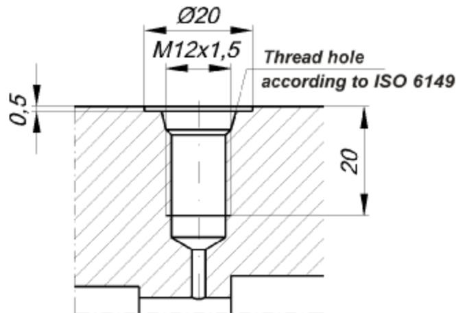
Figure 11: Dimensions of the reference measuring tap
