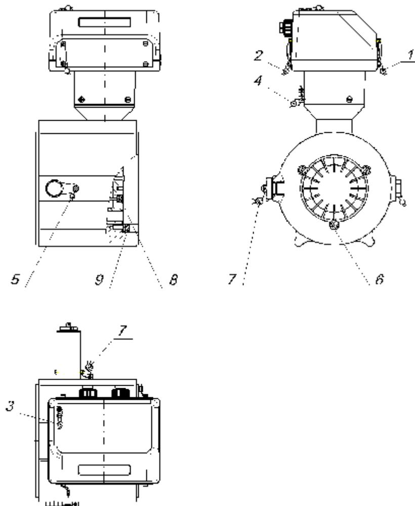
Figure 21: Seal positions of the quantometer CPT
