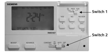
**Switch (1)** Programming switch. When all programming has been done this switch must be in Run
