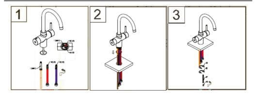
1. Assemble pipes to the underside of tap as marked:-
