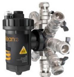
Servicing the intaKlean 2 is quick and easy and can be done without having to drain down the system. Simply close the full bore isolating valves, remove the magnetic core from the filter and open the drain plug. Once the filter has been drained, the screw cap and non ferrous filter can be easily removed for a comprehensive service. The filter pot has a fluid volume of 500ml - ideal for chemical dosing.
