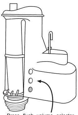
Press flush volume selector firmly into position to close the required holes.
