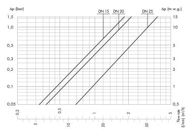
Recommended flow rate values to ensure stable operation and an accuracy of  $\pm$  2 °C
