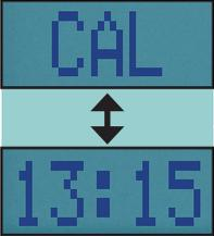
Display alternates between calibration due symbol & current time
