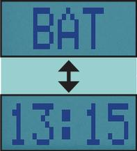
Display alternates between low battery symbol & current time
