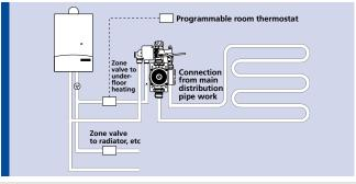
The pipe supplying the ZRU should be connected to the main boiler distribution pipe prior to the connection of other zone valves.
