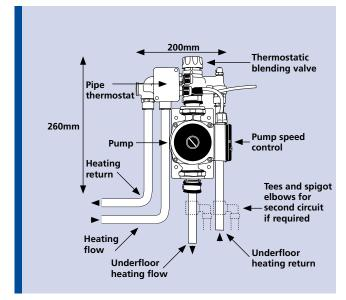
The ZRU simply connects to the existing heating system providing:
