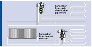
The diagram above shows the ZRU connected to operate with the boiler on/off firing. Due to the quick response of low mass systems (Overlay<sup>™</sup>, Overlay<sup>™</sup> Lite, MHP, etc) this is likely to be suitable. Using this method for solid floor installations may require the timings of the existing heating to be altered to allow the underfloor heating system to reach comfort temperature.
