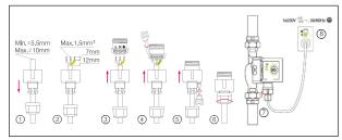
Connect the pump to the electrical supply in the order shown above
