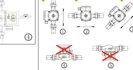
4.2 The control panel can be oriented in 2 of the 4 positions shown below.
