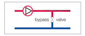
If all the thermostatic radiator valves in the system are closed, a bypass valve allows water to continually circulate eliminating unnecessary heat and pressure build up.
